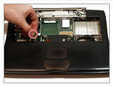
• Disconnect the wide orange cable that connects the airport card slot to the logic board.
