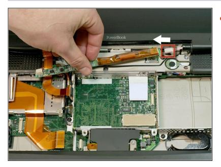
• Disconnect the white inverter cable from the right end of the board
