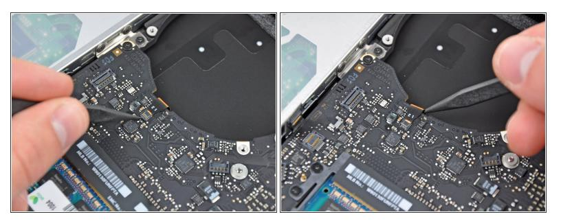
Use the tip of a spudger or your fingernail to flip up the retaining flap on the keyboard backlight ribbon cable socket.
