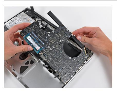
Carefully lift the logic board assembly from the left side and work it out of the upper case, minding the
