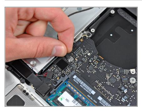
Disconnect the iSight cable by pulling its connector toward the optical drive opening.
