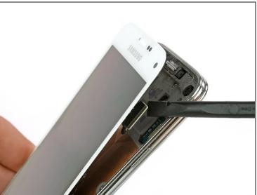
$\triangle$  Keep the top portion of the display assembly next to the frame.
