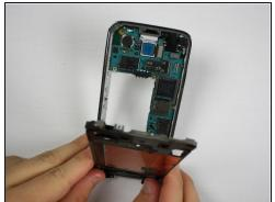
$\triangle$  Spread pressure out evenly to avoid damage or bending of the midframe.
