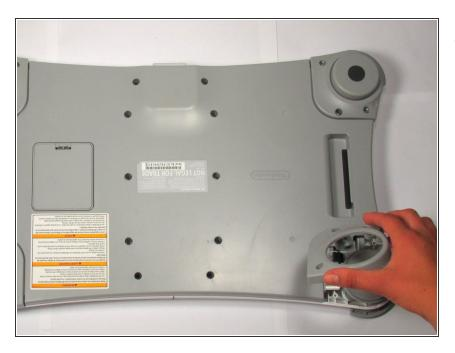
Remove the gray plastic ring from the actual foot by lifting it up.
