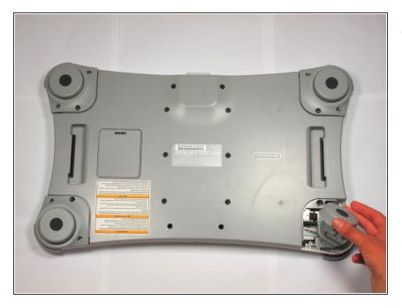
Separate the loose foot from the device by lifting it up.
