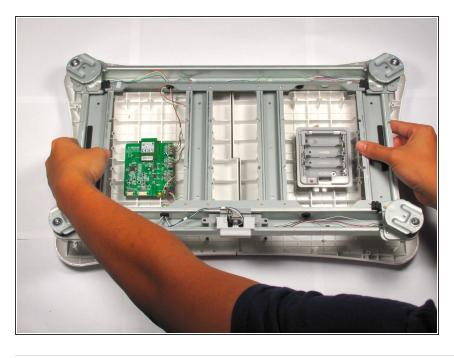
Lift the frame, circuit board, and power supply out of the front case.
