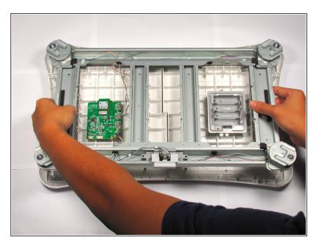
Lift the frame, circuit board, and power supply out of the front case. These components are all connected.
