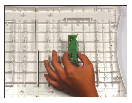
• Lift out the power supply. It is not screwed in.
