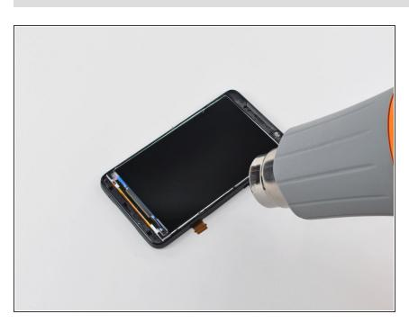
Use your heat gun to soften the adhesive under the LCD panel along its right edge.
