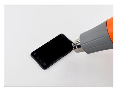
Use a heat gun to soften the adhesive along the right side of the front glass panel.
