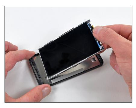
Lift the LCD panel assembly out of the inner case.
