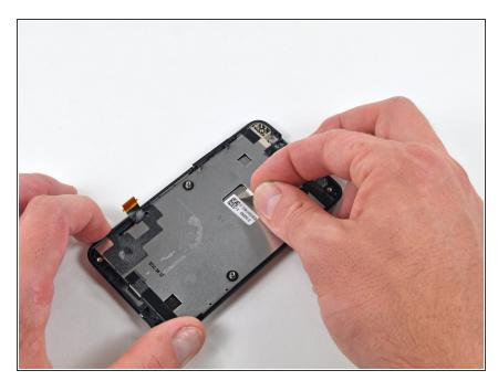
Peel the piece of tape connecting the underside of the LCD metal tray to the bottom of the inner case.
