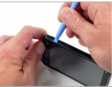
Insert the iPod opening tool between the front panel and its plastic surround and pry up at several points along the left edge of the Evo.
