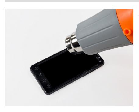
Use a heat gun to soften the adhesive along the left side of the front glass panel.
