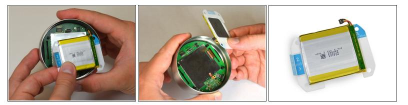
Grasp the battery with your fingers and pull directly away from motherboard to separate the battery from the display.
