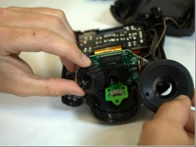
Once the device is open, remove the lens tunnel, then twist the lens to unscrew it from the camera.
