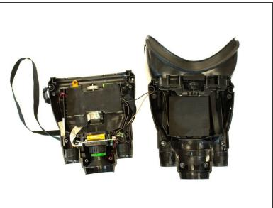
Remove the six silver 11.4 mm Phillips #0 screws and pry open the device, using the plastic opening tools if necessary. To do this, locate the groves running along the side of the entire device and wedge it open.
