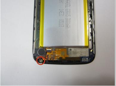
• The microphone is located at the rear-lower-left corner.
