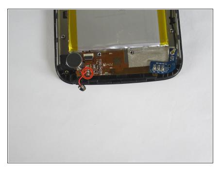
Solder the new microphone in the same spot. The black wire will go in the lower spot and the red wire in the upper spot. To reassemble your device, follow these instructions in reverse order.
