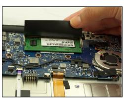
Locate the RAM under a black flap alongside where the laptop screen and device body meet.
