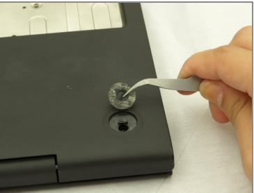
• Using a pair of tweezers, remove the two rear rubber feet to expose two hidden screws.
