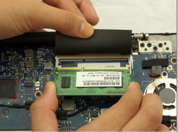
• Use two fingers to slide the RAM out at the angle that it has been released.
