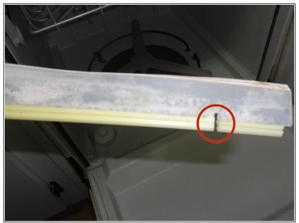
(i) Note that when installing the new seal there is an alignment tab located on the right hand side of the dishwasher (your right while facing the dishwasher). This tab needs to fit into the existing slot. If you have difficulty aligning this tab, you can remove the lower dishwasher rack to get a better view of the bottom side of the door.
