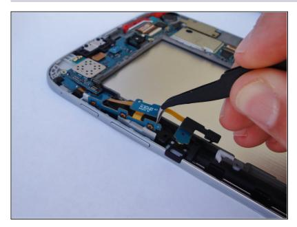
Using tweezers, pull the part of the cable that is located behind the volume buttons out of the slot.
