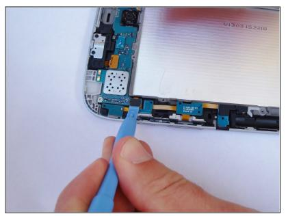
Disconnect the black connector by pulling up using a plastic opening tool underneath the edge. This connection attaches the power/volume cable to the mother board.
