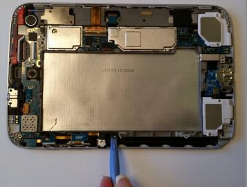
• Gently pry the lower edge of the cable off the plastic stud just above the stylus opening.
