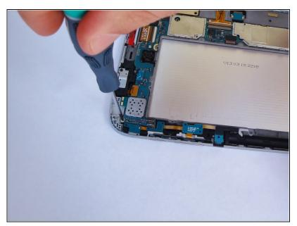
Remove the 3-mm screw holding the upper left corner of the main board using a Phillips#00 screwdriver.
