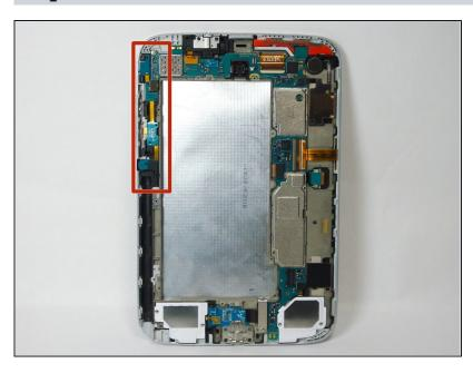
The volume and power buttons are joined together on a common strip, so you are replacing both simultaneously.
