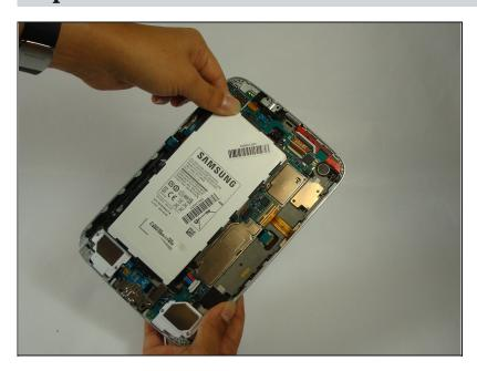
• Lift the top left corner of the battery up by the black tab.
