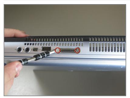
Using a flathead screwdriver, remove two screws on the leftside panel of the laptop.
