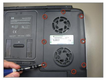
Loosen the eight Phillips screws around the plate to remove it.
