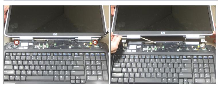
To begin disconnecting the monitor, remove two screws.
