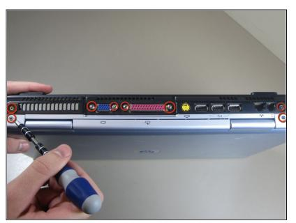
• Remove eight screws from the back panel of the laptop.
