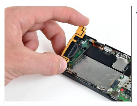
• Carefully lift and remove the speaker assembly up out of the phone.
