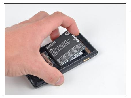
Grasp the upper left corner of the battery and lift it out of its housing.
