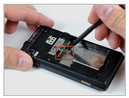
Insert the flat end of a spudger and pry downwards to release the plastic tab holding the rear case to the motherboard screw.
