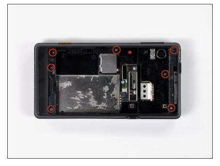
Remove the seven 5.5 mm T5 Torx screws securing the rear case to the inner case.
