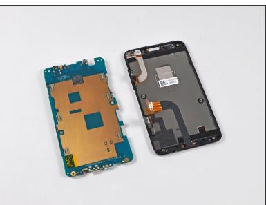
After disconnecting ribbon cables for the display, digitizer, and front camera, the logic board can be removed from the front half of the Evo.
