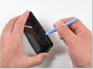
We delve deeper into the Evo 4G by removing six T5 Torx screws and carefully prying off the internal frame with an iPod opening tool.
