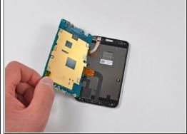
A small Phillips screw near the top left corner of the Evo is all that keeps the left side of the logic board snug in its cradle.
