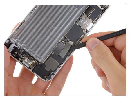
Pry the vibrator connector cable up from its socket on the logic board with the flat end of a spudger.
