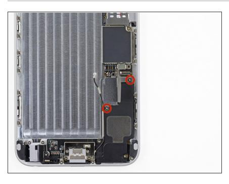
Remove the two 2.5 mm Phillips #00 screws securing the vibrator to the rear case.
