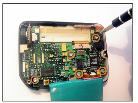
Use the T9 Screwdriver to remove the five visible screws: Top right, bottom right, middle center, bottom center, bottom left.
