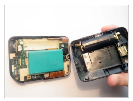
• Remove the backside of the device and set aside for later use.
