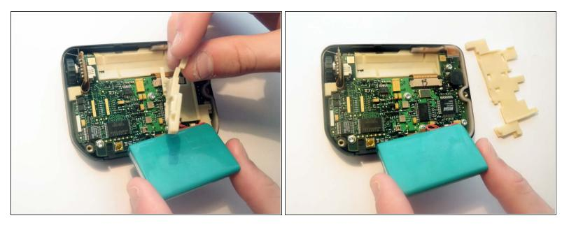
• Remove the rubber placement pad that sits under the battery and set aside for later use. Gently fold back the battery, making sure the small plug connecting the battery to the logic board remains intact. Extra care should be taken as this part is quite delicate and easy to damage.
