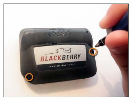
Use a T9 Screwdriver to unscrew the two screws on the backside of the BlackBerry, one on the bottom left and one on the top right.
