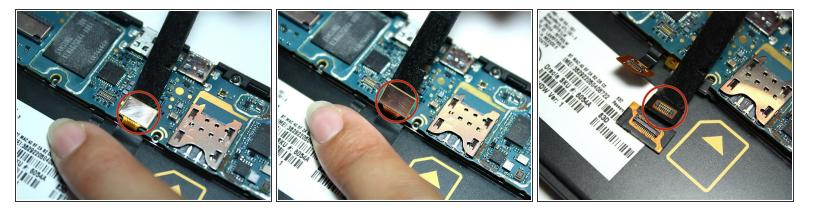
Repeat the same step for the final ribbon cable located under the larger one.
