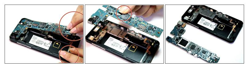
Now that all of the ribbon cables have been disconnected, carefully lift the motherboard from its housing with your thumb and index finger. Start lifting the motherboard from the bottom and work your way to the top. Hold down the phone with your other hand so you have a better grip on the device. Once removed, turn the motherboard over.
