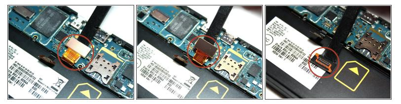
Then, use the nylon spudger to lift up and open the other gold ribbon cable located behind the previous one.
