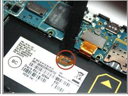
Next, use the nylon spudger to open gold ribbon cable adjacent to the battery housing.
