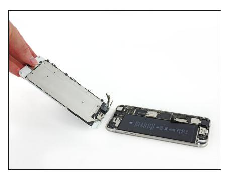
Remove the front panel assembly from the rear case. To reassemble your device, follow these instructions in reverse order.
