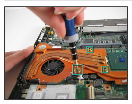
Remove the three screws on the fan.
