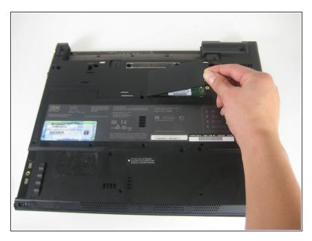
Remove the extra RAM cover, by lifting where the screw was and pulling out.
