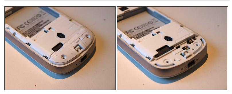
Remove the antenna (use the little gap at the top).
