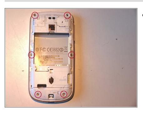
Unscrew the six screws with a Torx
