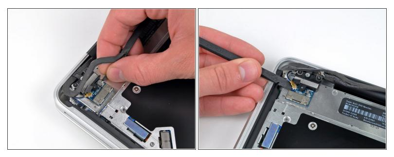
• Disconnect the Bluetooth cable by pulling the male end straight away from its socket.
