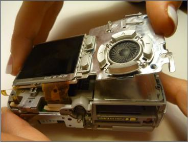
• To check that all screws are removed from the exterior side panel, gradually slide and lift no more than 3cm away from the camera internal component body.
