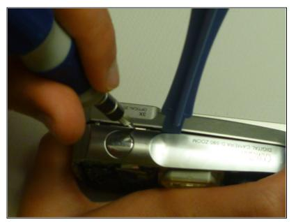
Using an iFixit opening tool, pry the backplate from the camera internal housing component.
