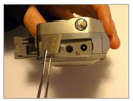
• Using tweezers, lift the rubber plate to expose the ports.
