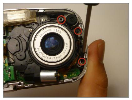
Using a Phillips #00 screwdriver, remove three screws fastened to the camera backplate edge.
