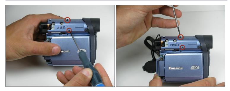
• Remove the indicated 4.5mm screws from the LCD side of the camera.
