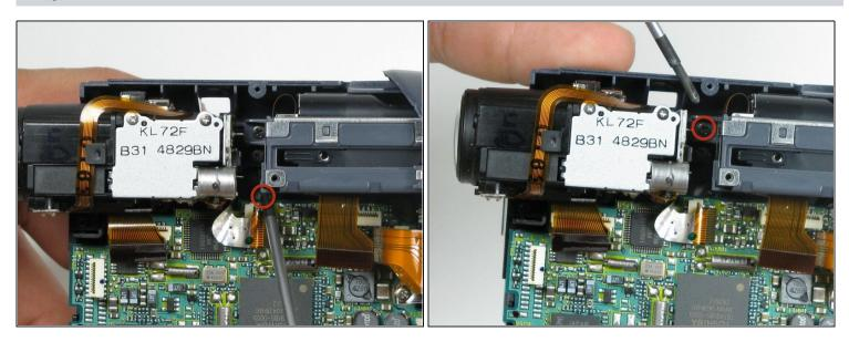
• Using #00 phillips screwdriver, remove two 4.5mm black screws holding lens in place.
