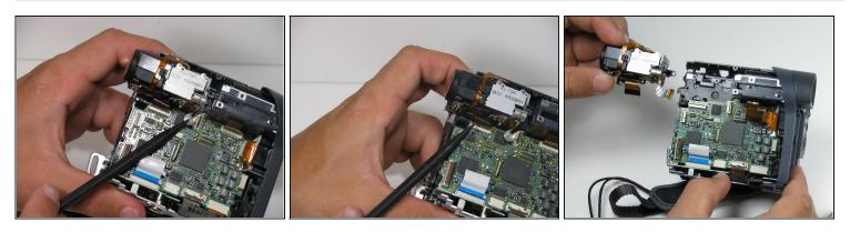
• Careful that both lens ribbon cables are removed from logic board, remove lens.
