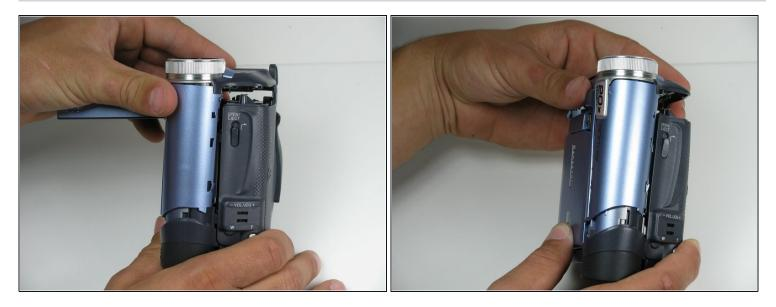
(i) Carefully remove the front cover from the body of the camcorder.
