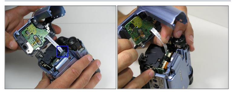
• Using your fingers, carefully pull the ribbon cable away from the logic board.
