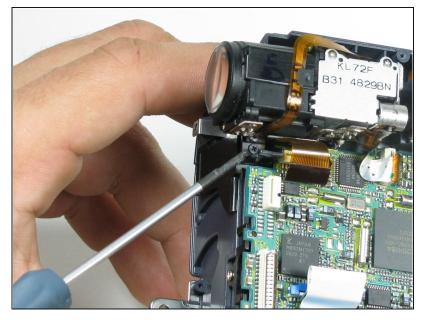
• Remove third 4.5mm lens mount screw near front of camera.
