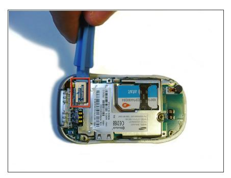
Detach the tab from the logic board shown by using the lpod Opening Tool
