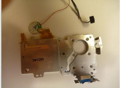
Gently lift the speaker from the LCD screen fitting.
