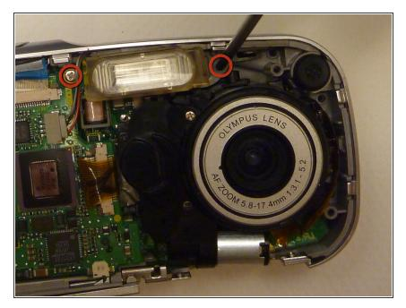
Using a Phillips #00 screwdriver, remove the two camera flash screws secured to either side of bulb housing component.
