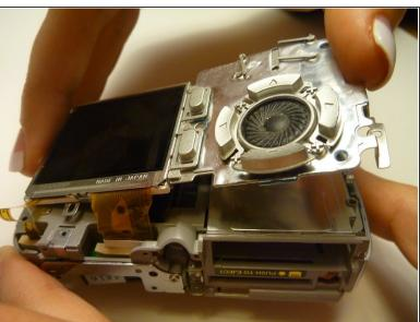
To check that all screws are removed from the exterior side panel, gradually slide and lift no more than 3cm away from the camera internal component body.
