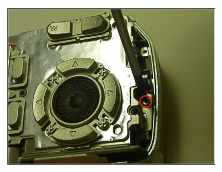
Remove one screw Phillips #00 from the right side of the LCD screen camera internal housing component.
