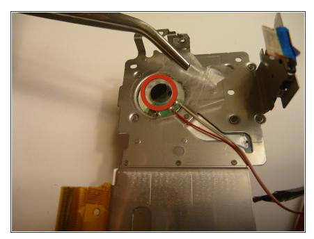
Using tweezers, gently lift and remove the clear tape covering the speaker.
