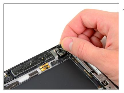
Carefully peel the rubber cover off the metal camera retainer and remove it from the iPad 2.
