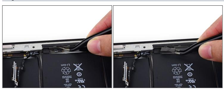
• Use a set of tweezers to remove the foam block from between the rear case and the upper component board.
