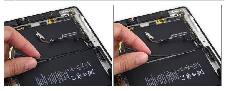
• Lift the end of the upper component board cable up off of the adhesive holding it to the rear case.
