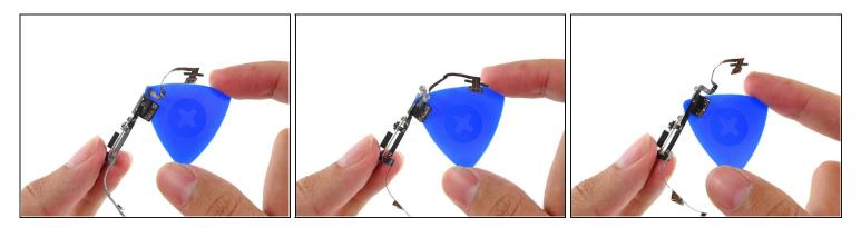
• Slide the opening pick under the remaining portion of the rotation lock/silent switch to peel it up off the button bracket.
