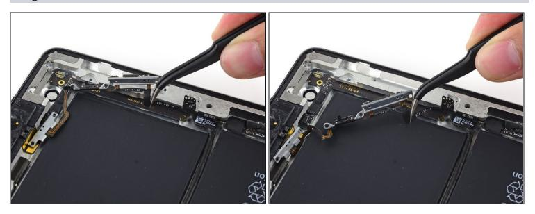
• Carefully peel the volume rocker portion of the button cable away from the rear case.
