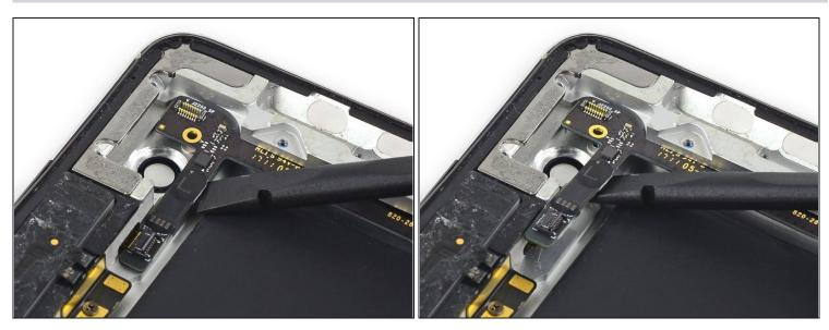
• Insert a spudger under the GPS connector end of the upper component board and lift it up off of its adhesive.
