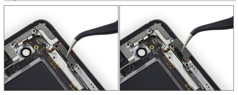
• Remove the metal bracket securing the rotation lock/silent switch.
