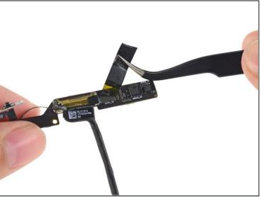
• Peel the tape covering the button cable connector off of the upper component board.
