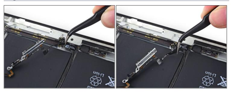
Gently peel the last horizontal portion off of the rear case.
