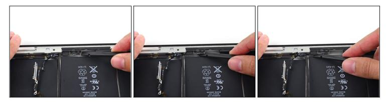
• Insert a spudger under the end of the upper component board and gently slide it toward the volume rocker to free the board from adhesive.
