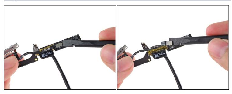
• Lift the button cable connector straight up off of its connector on the upper component board.
