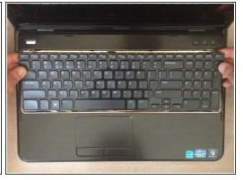
By using cutter, carefully lift up the one side of the keyboard and start opening the locking clips.
