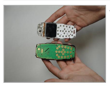
Pry the layers apart. The LCD and plastic layer will lift out as one piece.
