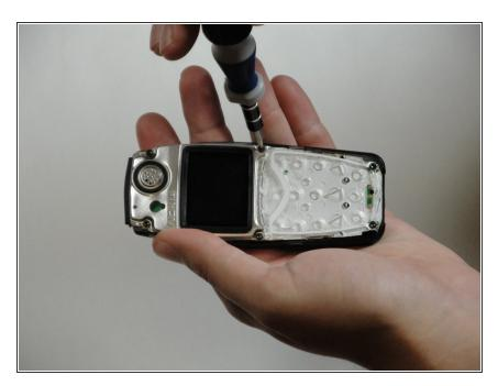
Unscrew the six screws with a Torx screwdriver (six-pointed star shaped bit).
