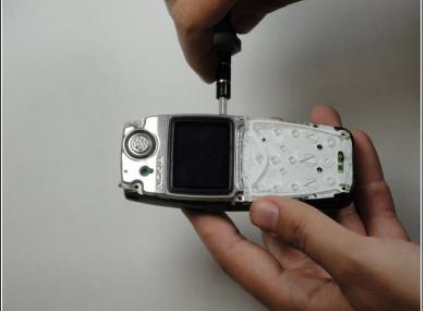
Insert a flat screwdriver between the black body and plastic layer.
