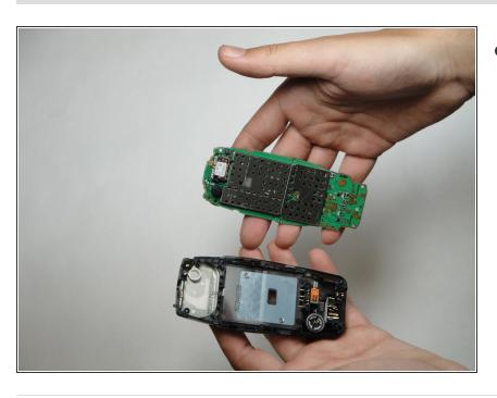
With the screws removed, the logic board can then be lifted out of the body by hand.
