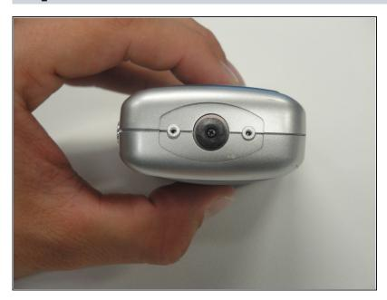
Remove the 5 mm screw and cap that were underneath the camera strap eyelet.
