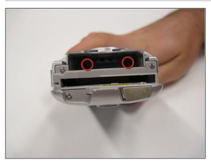
• Remove the two 4.5 mm screws that sit inside the battery slot.
