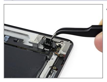
• Remove the plastic camera bracket.
