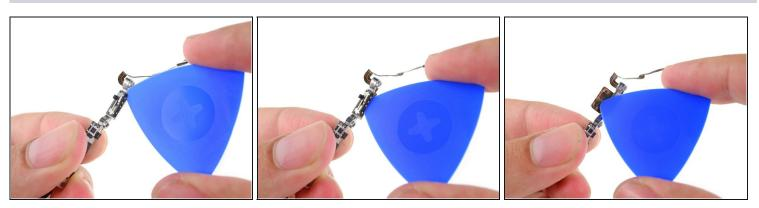
• Insert the point of an opening pick between the rotation lock/silent switch and its bracket to sever the adhesive there.
