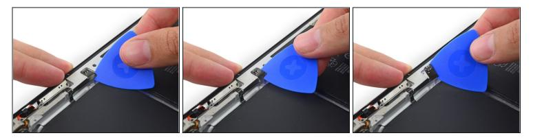
• Use the point of an opening pick to gently peel the Smart Cover sleep/wake sensor up off the rear case.
