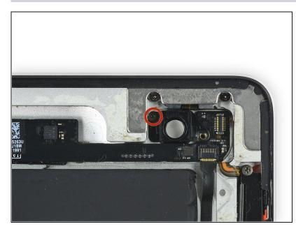
• Remove the single 2.0 mm Phillips #000 screw securing the camera bracket.
