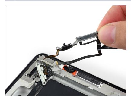
• Remove the button cable assembly from the rear case.
