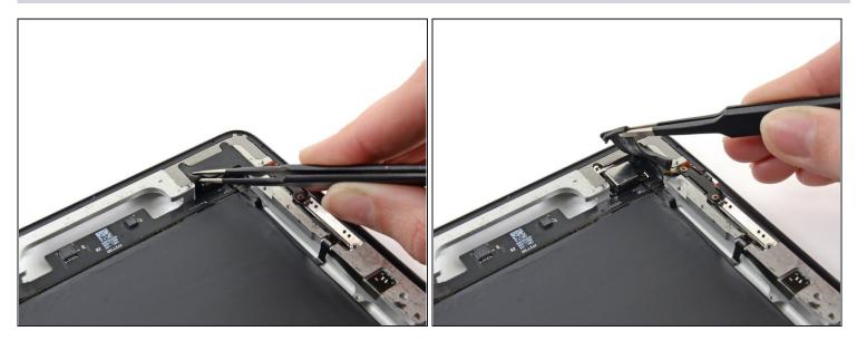
• Use a pair of <u>tweezers</u> to remove the rubber cover up off the rear-facing camera housing.
