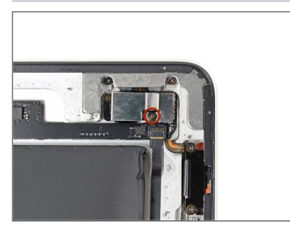
• Remove the single 3.3 mm Phillips screw from the rearfacing camera metal retainer clip.
