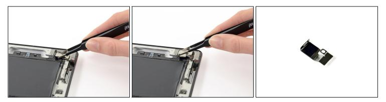
• Lift the rear-facing camera metal retainer clip straight up from its recess in the rear case.
