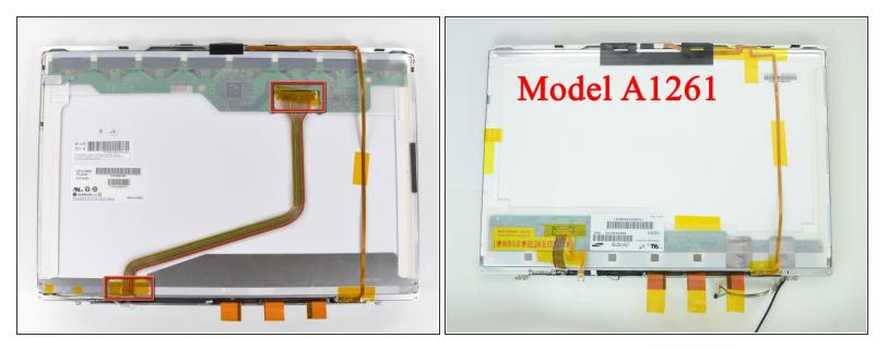
• Remove the two pieces of tape securing the display data cable to the LCD.
