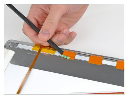
Use the flat end of a spudger to carefully peel off the three antenna straps stuck to the lower edge of the LCD.
