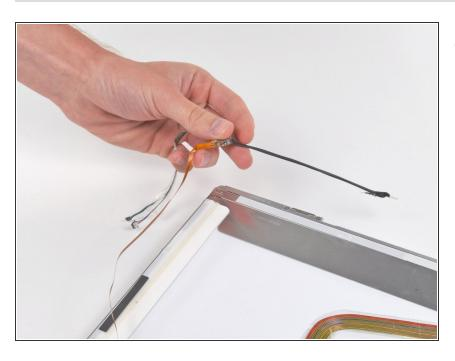
• Remove the inverter/antenna cables from the display.
