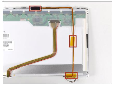
Remove the three pieces of tape securing the camera cable to the display assembly.
