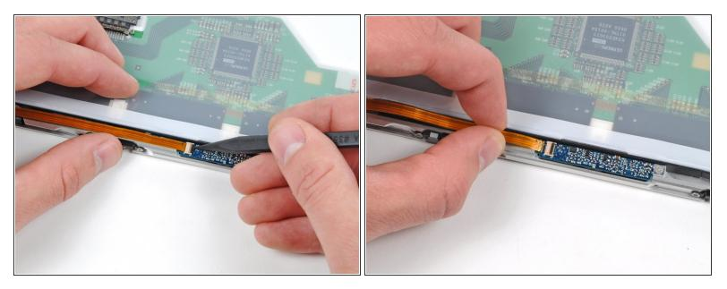
• Use the tip of a spudger or your fingernail to flip up the ZIF retaining flap on the camera cable socket at the edge of the camera board near the top center of the front display bezel.
