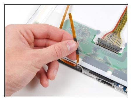
Peel the camera cable off the foam tape along the top edge of the display.
