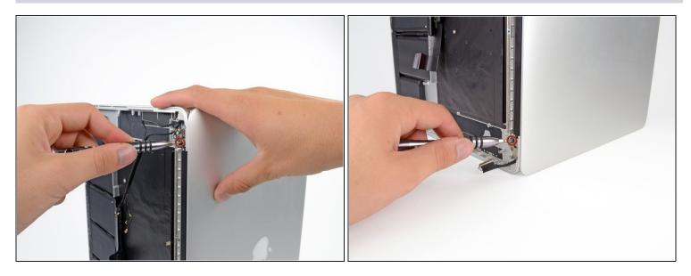
(i) Open the device between 90 and 100 degrees, then rest it on its side.
