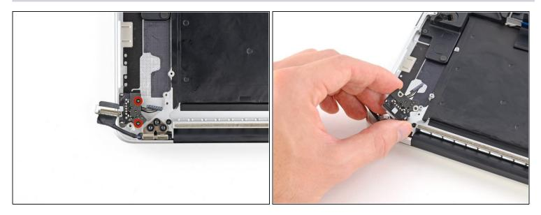
Remove the two 4.0 mm T5 Torx screws securing the MagSafe DC-In board to the upper case.
