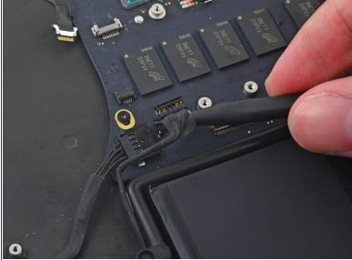
Use the tip of a spudger to lift the right speaker connector straight up out of its socket on the logic board.
