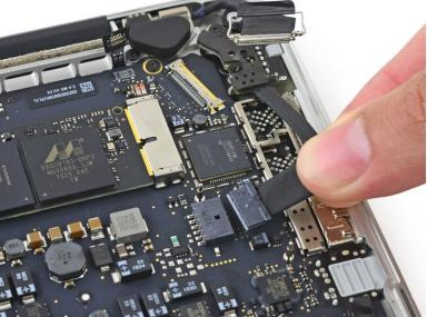
Carefully pull the DC-In board connector straight out of its socket on the logic board.
