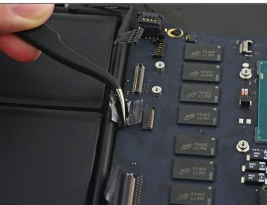
Pull the trackpad ribbon cable straight out of its socket on the logic board.
