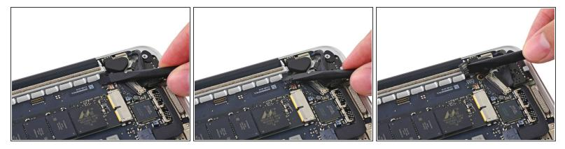
Use the flat end of a spudger to disconnect the keyboard backlight cable and bend it up out of the way of the logic board.
