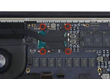
Use the flat end of a spudger to peel the four foam stickers off of the heat sink screws.
