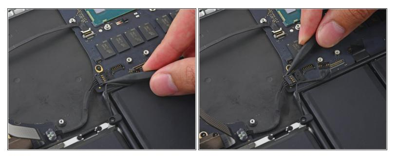
With the tip of a spudger, push on either side of the I/O board connector to walk it out of its socket on the logic board.
