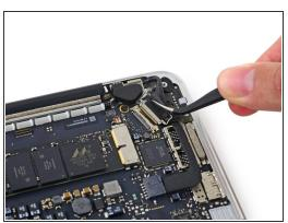
Grab the black plastic tab to flip the display cable connector open and pull it straight out of its socket on the logic board.
