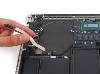
Lift the logic board end of the I/O board cable straight up to bend it out of the way.
