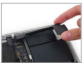
• Lift the corner of the left speaker up and slide it toward the battery to remove it from the upper case.
