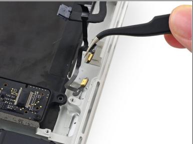
Pull the dual microphone cable assembly up and toward the logic board recess to remove it from the upper case.
