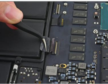
Pull the keyboard cable straight out of its ZIF socket on the logic board.
