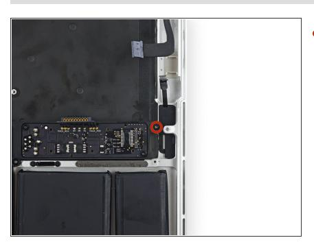
Remove the single 3.7 mm T5 Torx screw securing the case-edge of the battery contact board.
