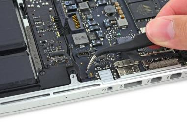
(i) If necessary, peel back any tape covering the microphone cable ZIF connector.
