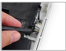
Insert the tip of a spudger under the battery-side portion of the microphone ribbon cable and slide it toward the screw post to free it from the upper case.
