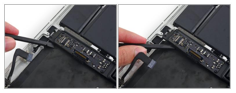
Use the flat end of a spudger to wedge the battery contact board up slightly to allow room to extract the dual microphone assembly.
