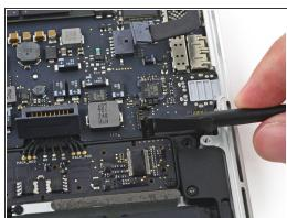
Wedge the flat end of a spudger under the left speaker cable near the connector and lift it straight up out of its socket and fold it out of the way.
