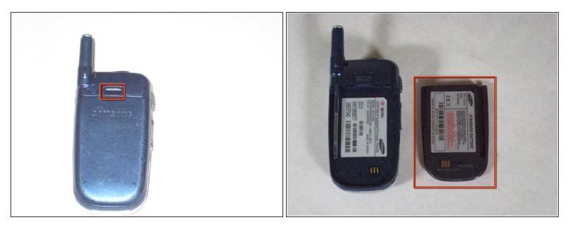
• Push open the latch and remove the battery.
