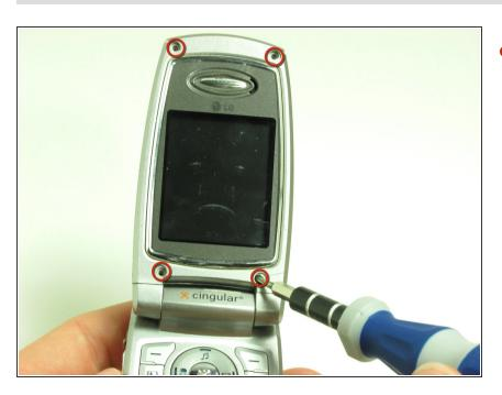
Using a T6 Torx screwdriver, remove all four screws.
