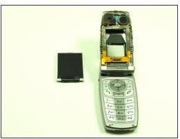
Carefully lift the LCD screen and peel it from the gold ribbon. The sticky connection runs all the way around the LCD screen.
