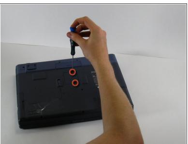
Remove the two clock battery screws with the screwdriver.
