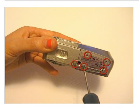
Remove five baseplate screws using a Phillips #00 screwdriver.
