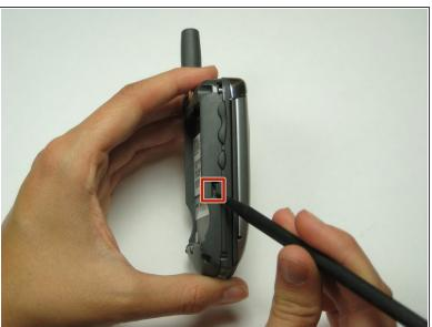
Simultaneously press the highlighted buttons on both sides of phone.
