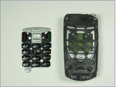
To replace keypad buttons, lift off white tray containing buttons.
