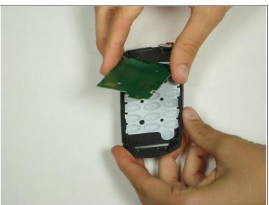
Once logic board is removed lift the green keypad sensor for the front plate.
