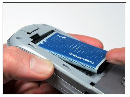
Remove the battery from the battery housing by flipping up the top of the battery.
