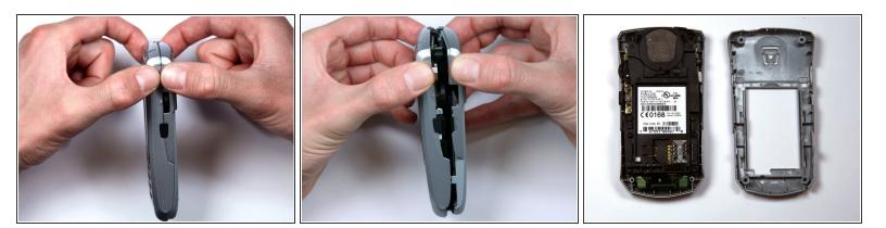
(i) The keypad cover may fall out of the housing when prying the housing apart.
