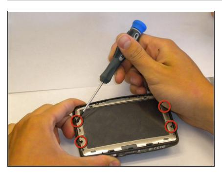
Remove the four Phillips #00 screws around the edge of the screen.
