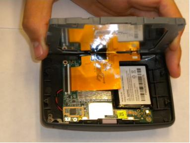
Lifting from the upper edge of the screen, tilt the screen away from the device.
