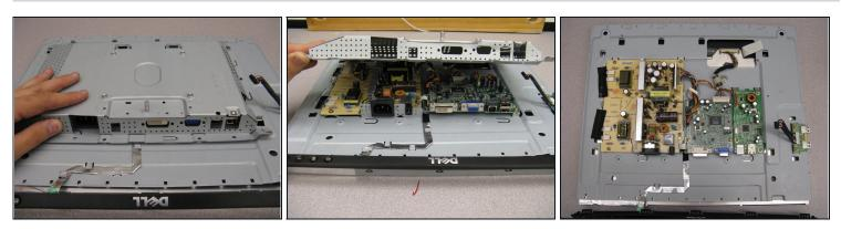
• Lift up on the back panel to remove it from the rest of the monitor.
