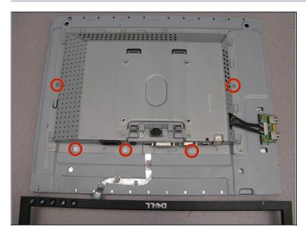
• Remove the five 5 mm Phillips #2 screws from the back panel.
