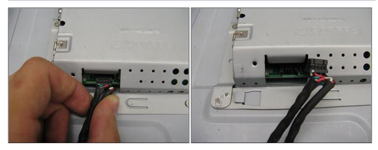
• Disconnect the USB ports by gentling grasping and pulling on the connector.
