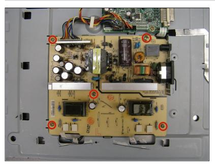
Remove the five 7 mm Phillips #2 screws from the power supply board.
