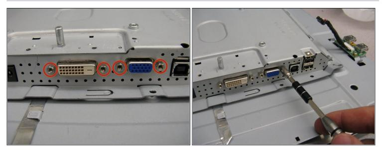
• Use a 5 mm nut driver to remove the four 12 mm standoff screws securing the video connectors to the panel.
