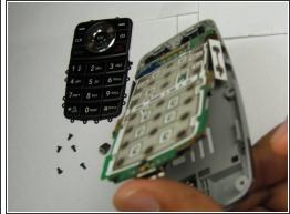
Pry open the phone and remove the keypad and logic board.
