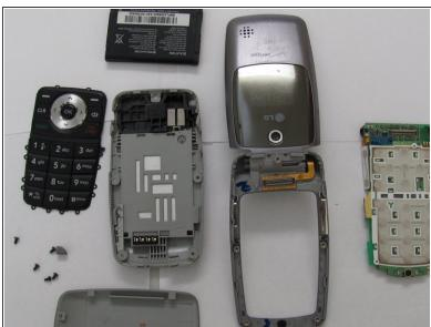
Lay out and organize the parts of the phone. You can now put the inner parts of the phone into the new case.
