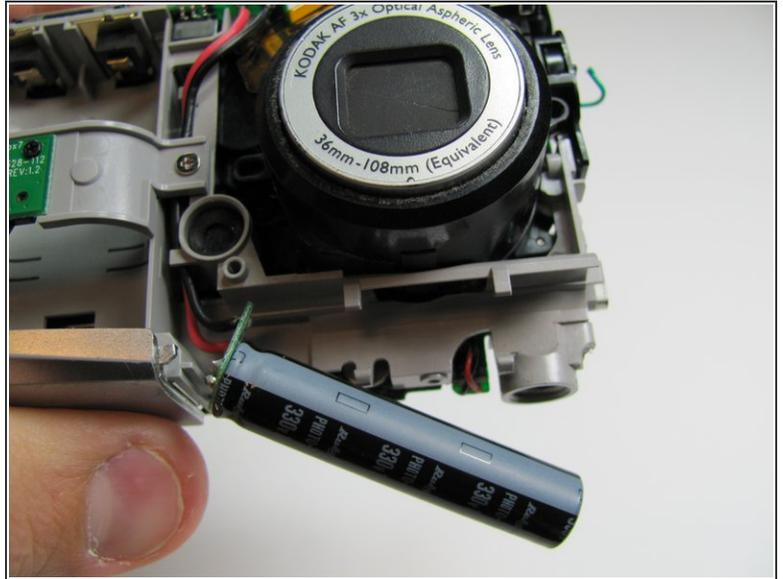
⚠ To avoid an electric shock, do not touch capacitor.
