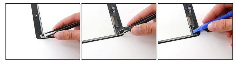
(i) In this step you will be transferring the smart cover magnets to the **NEW** front panel assembly.
