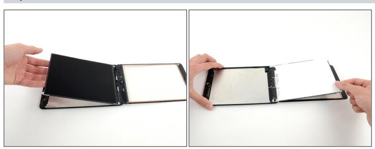
• Flip the LCD over and rest it on top of the front panel glass.
