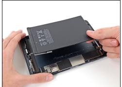
Lift and remove the battery from the iPad.
