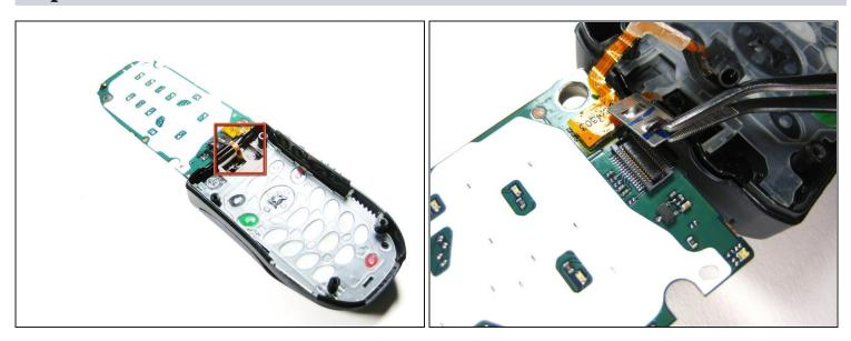
• Using <u>tweezers</u>, carefully pull off the connector shown.
