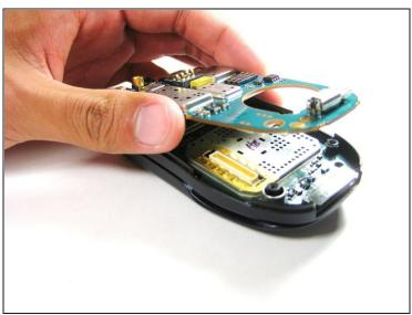
• Lift the first logic board off of the rest of the device.
