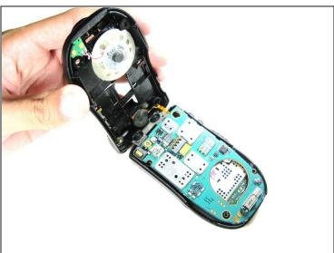
$\triangle$  DO NOT force the cover off as it could damage the ribbon cable!
