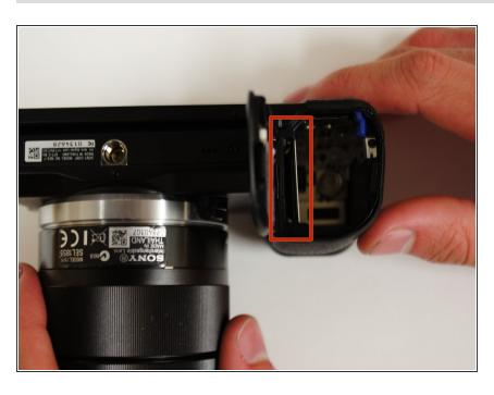
To the left of the battery compartment, the SD card needs to be pushed down slightly with your
