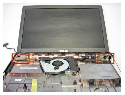
Locate both of the hinges that connect the monitor to the bottom plate cover.
